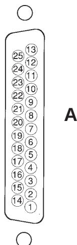
Diagram showing back of typical DB-25 connector plug, with pin numbers oriented as they would be seen from rear of console.
